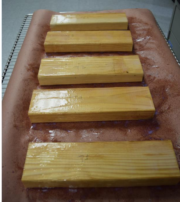
Figure 5 Five 2x4 Wood Specimens Right after Coatings Applied
