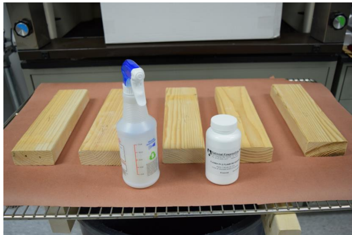
Figure 4 Five 2x4 Wood Specimens Right Before Coatings Applied
